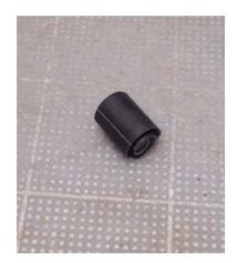
Roll the black strip and then cut the individual segments, then roll each segment into a very thin cylinder of approximately 2 mm in diameter. In total there are 8 pins for all the legs.
