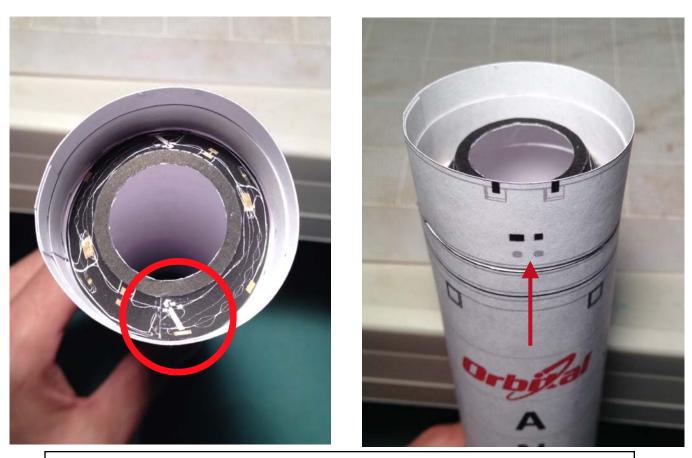
Align the white vertical drawing on the Motor Cone with the 4 small squares on the side of the rocket (arrow)
