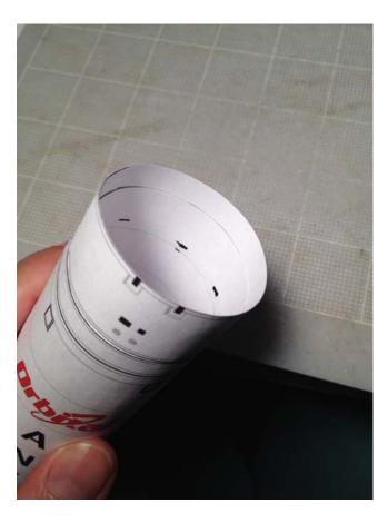
In order to insert the Motor Cone Support Rings, one must draw some markings 18 mm down from the top of the rocket tube as shown.
