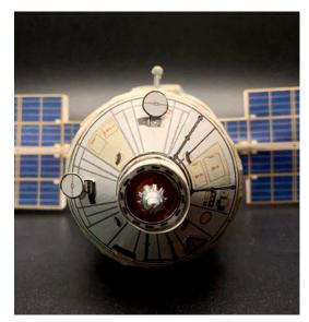
This photo shows the probe connector that can be removed in order to put the connecting cylinder (see above). The probe connector piece should not be glued. It's for flight configuration only.
