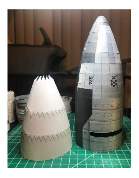
The nosecone interior consists of three skin sections that when glued together makes a single piece, as seen on the photo on this photo. This step is the same for all of my Starship models, whether you're building the early ones or the current Starships.
