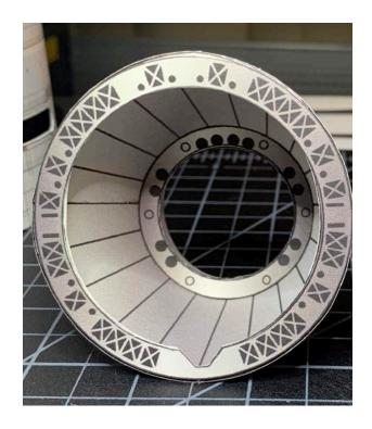
This COPV enclosure is the same as the Early configuration type. The difference is the position of the COPVs. This photo is from my test model which at the time had erroneously 12 tanks.
