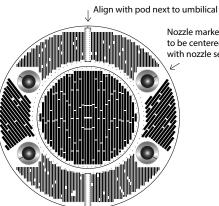
Nozzle marker line to be centered with nozzle seamline
